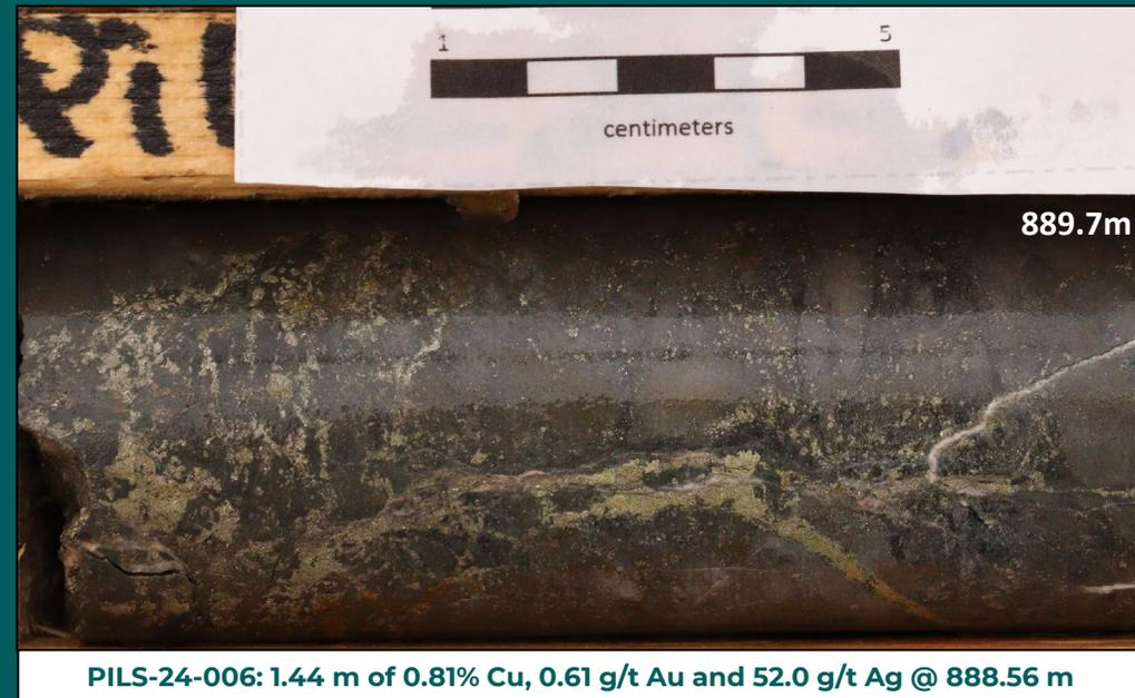
In 2024, the 2 holes were drilled at PIL South, totaling 1,759 m. The drillholes were designed to test favourable geology, and chargeability and resistivity anomalies deeper than past drilling.
